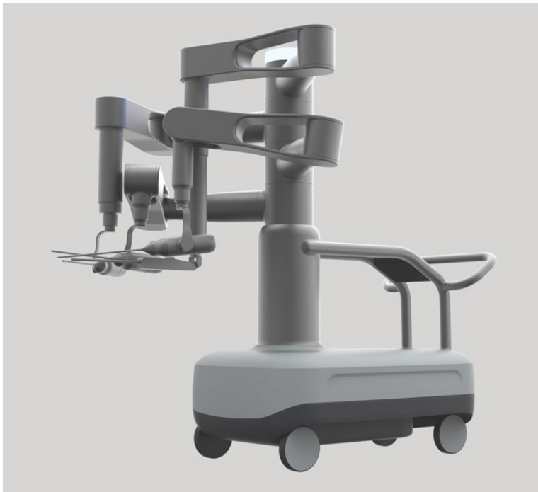
Figure 2: The Bitrack of Rob Surgical is the result of more than ten years of cutting-edge research in surgical robotics. Source: Rob Surgical
