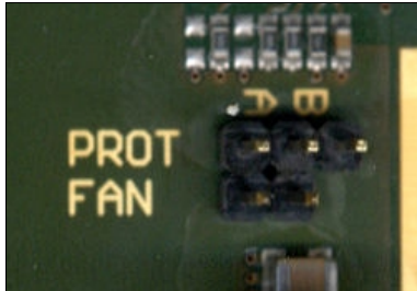
Figure 5: Jumpers PROT and FAN (detail, normal version)
