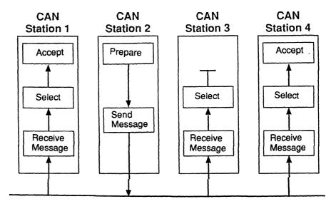
Broadcast transmission and acceptance filtering by CAN nodes
