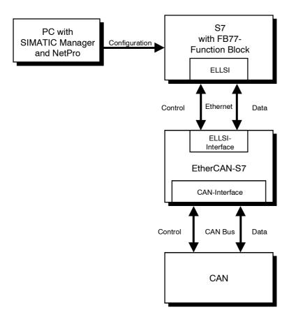
Fig. 1: Connection of Siemens-PLC S7 to a CAN bus via EtherCAN-S7
