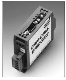
They are connected via 5-pin screw/plug connectors in Combicon design.
