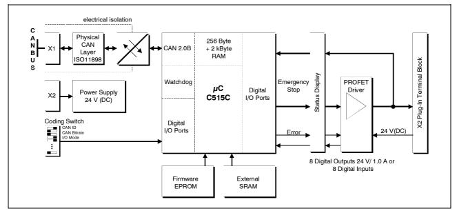
Fig. 3: Block-circuit diagram of the CAN-CBM-DIO8 module
