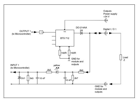
Figure 4.2.1: Schematic diagram of input and output circuits
