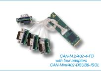
The adapter cable is included in delivery. The card length can be easily reduced. The CAN-M.2/402-4-FD-T variant is designed for use in the extended temperature range.
